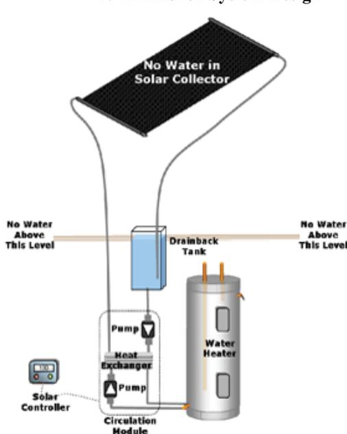
Figure 24. Drainback system "off"
