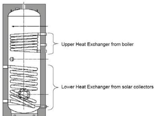
Figure 23. A two heat exchanger solar tank for installation with a heating boiler (Schüco)<sup>43</sup>
