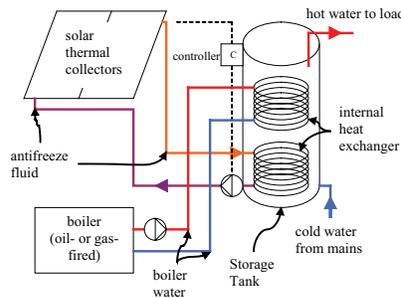
**Figure 10. Tank Design x4x - Double Heat Exchanger Tank**
