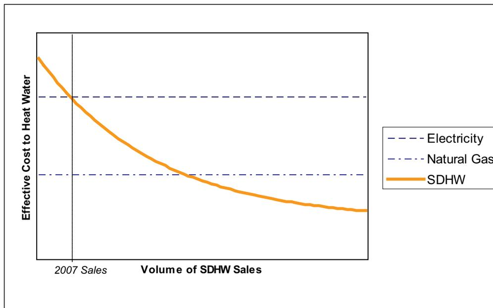
**Figure 3. Effective Cost to Heat Water with Solar, Electricity, and Natural Gas<sup>5</sup>**
