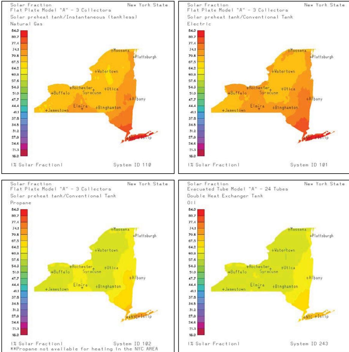
**Figure 12. Statewide Renderings of Highest Solar Fraction for each Fuel Type**
