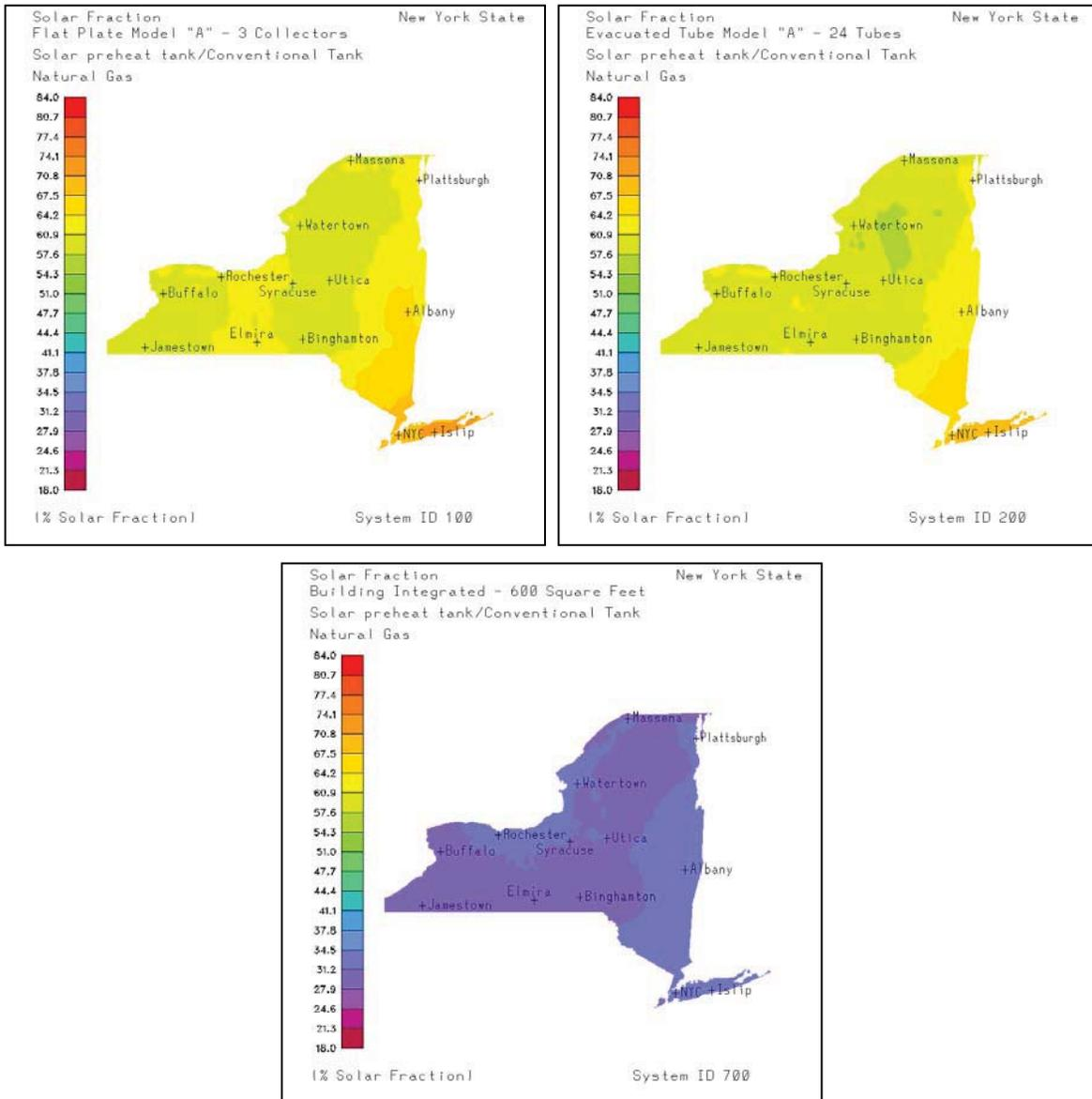
Figure 13. Statewide Renderings of Highest Solar Fraction for each Technology Type<sup>20</sup>
