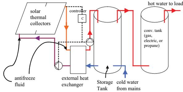
**Figure 8. Tank Design x2x - Solar preheat tank with External Heat Exchanger + Conventional Tank**
