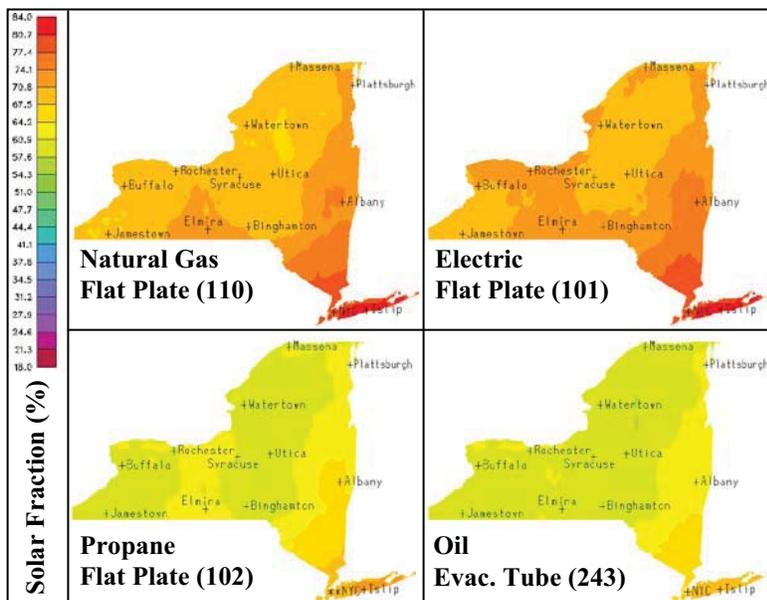
**Figure 1. Renderings of Solar Fraction for best performing systems of Each Fuel Type. (Maps for all systems analyzed are available at <http://sdhw.brightpower.biz>)**
