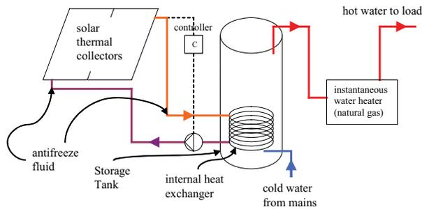
**Figure 7. Tank Design x1x - Solar preheat tank + Instantaneous (tankless) heater**
