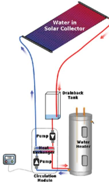
Figure 25: Drainback system "on"
