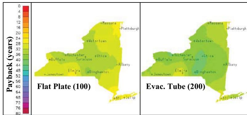
**Figure 4. Rendering of Simple Payback of best-in-class systems in two tank arrangement co-fired with natural gas**
