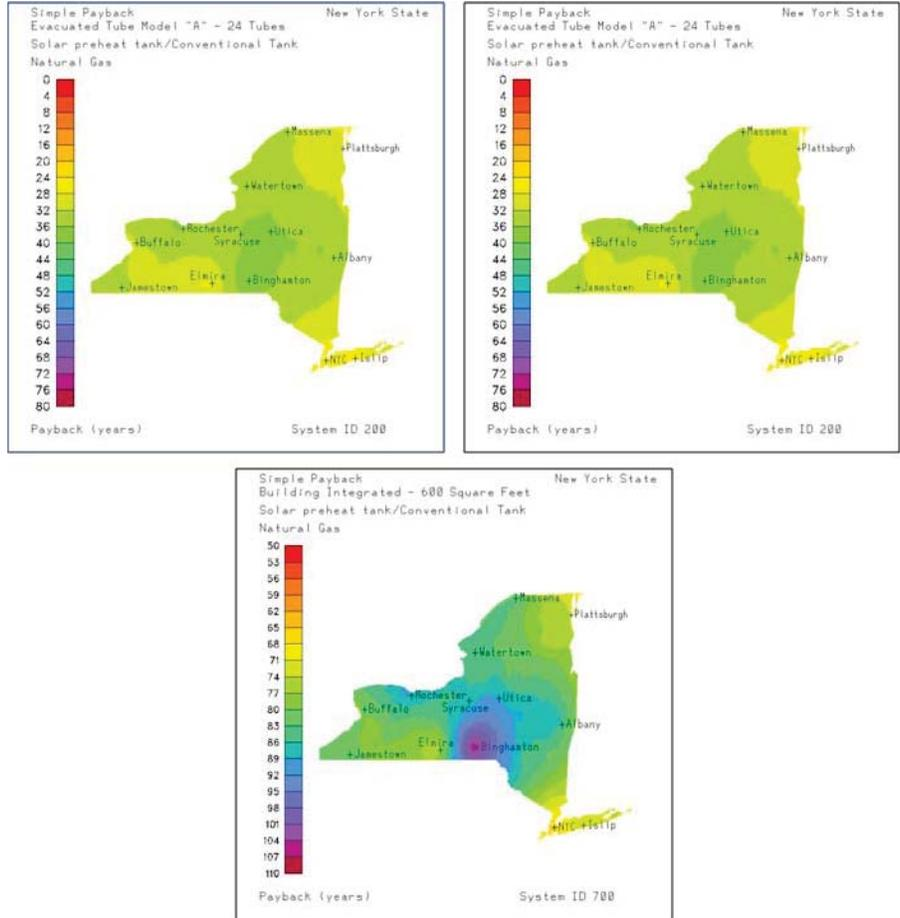
**Figure 21. Statewide Renderings of Shortest Payback Time for each Technology Type**<sup>27, 28</sup>
