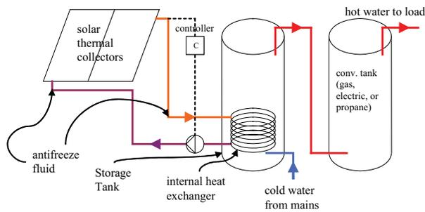
**Figure 6. Tank Design x0x - Solar preheat tank + Conventional tank**
