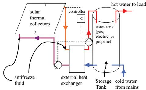
**Figure 9. Tank Design x3x - Conventional Tank with External Heat Exchanger**
