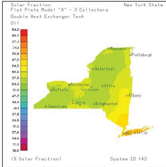
Figure 14. Rendering of System with Most Statewide Variability in Solar Fraction<sup>21</sup>
